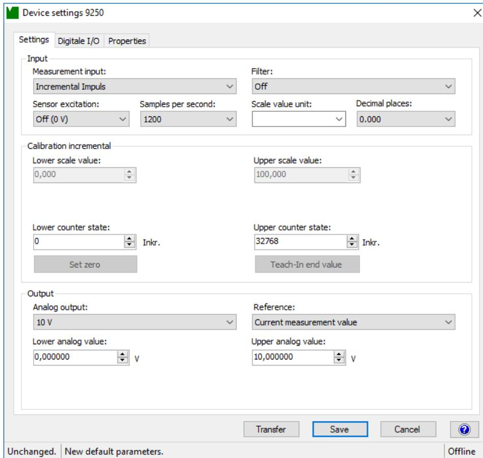
Diagram: 43 Device settings for the totalizing counter (Incremental Impuls mode)
