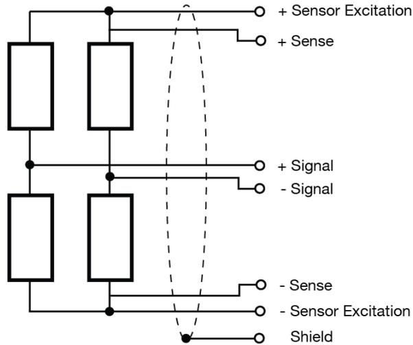
Diagram: 6 Strain-gage connection method
