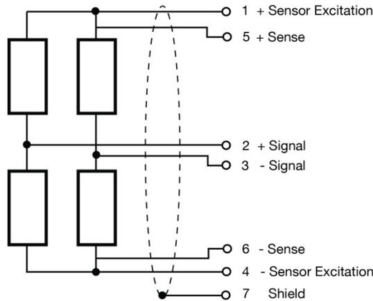
Diagram: 8 Strain-gage sensors with sense leads
