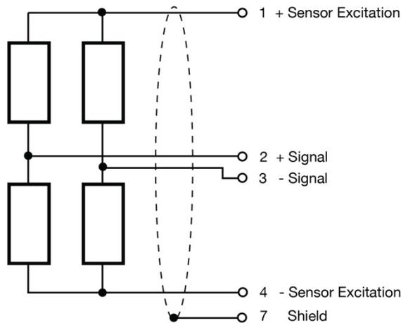
Diagram: 7 Strain-gage sensors without sense leads
