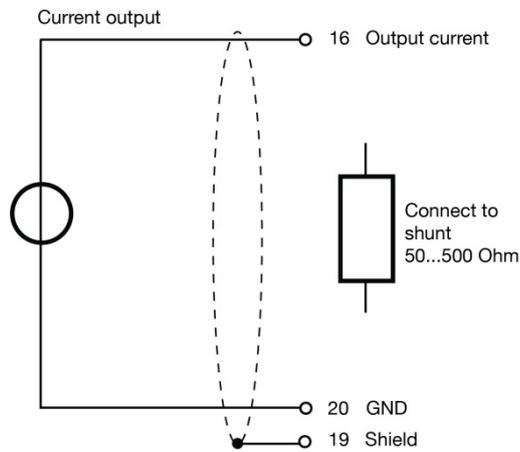
Diagram: 14 Terminal assignment for the current output
