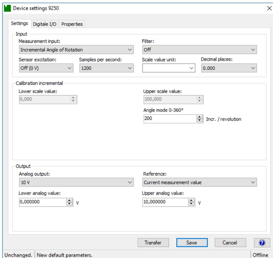
Diagram: 44 Device settings for 360° angle of rotation (Incremental Angle of Rotation mode)
