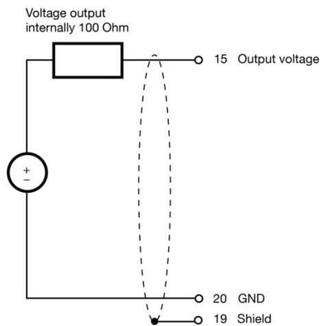
Diagram: 13 Terminal assignment for the voltage output
