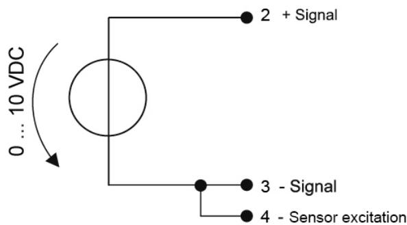
Diagram: 10 Transmitter with voltage output
