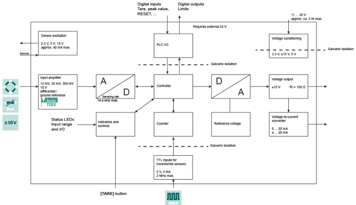
Diagram: 1 Block diagram of the 9250 instrumentation amplifier
